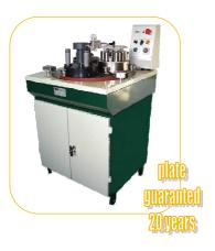
Machine for the lapping of samples and glass sample holders, and for the final lapping of thin sections. Comes with a sample holder for up to 12 sections, a control device, an automatic straightening system for the plate, a thickness measuring set and a first run set of consumables. 20 years of guarantee for the lapping plate.
